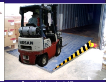
Form a bridge enable forklift to drive into container for loading-unloading of goods.
